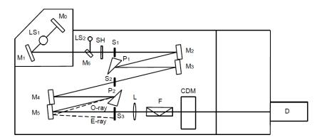
$M_0 \sim M_6$ : Mirrors O-ray : Ordinary ray LS<sub>1</sub> : Xenon lamp (for sample measurement) E-ray : Extraordinary ray
